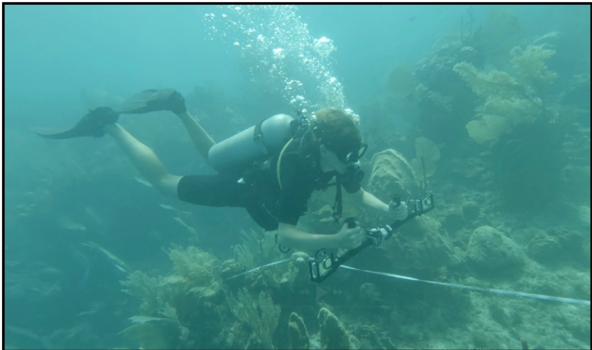
Figure 7: SVS survey for illustration, note that during an active SVS survey, the transect line would not yet be laid.
